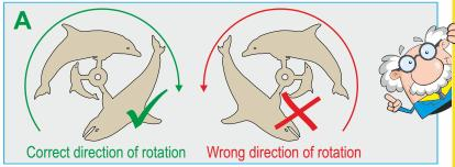
Screw the dolphin wheel (position it as shown in the picture) to the gearbox axle A with the M3 x 5 mm screw using the screwdriver. Secure it in place with the wood spanner to prevent it from turning. Then apply a thin layer of glue on the wave plate (where it is red in picture 2) and then glue it in the middle of the base plate. The 3 slots in the base plate must point forwards as in picture 3.
