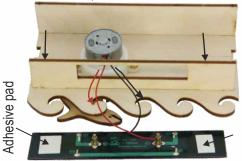
3 Feed the motor cable through the solar cell support and connect it to the solar cell. Press the button, push in the cable, release the button - job done. Red cable to "-", black cable to "+".
