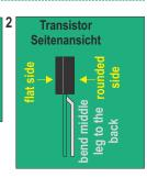
The feet on the transistors are very close. Therefore be very careful when soldering to avoid a short-circuit between the legs.
